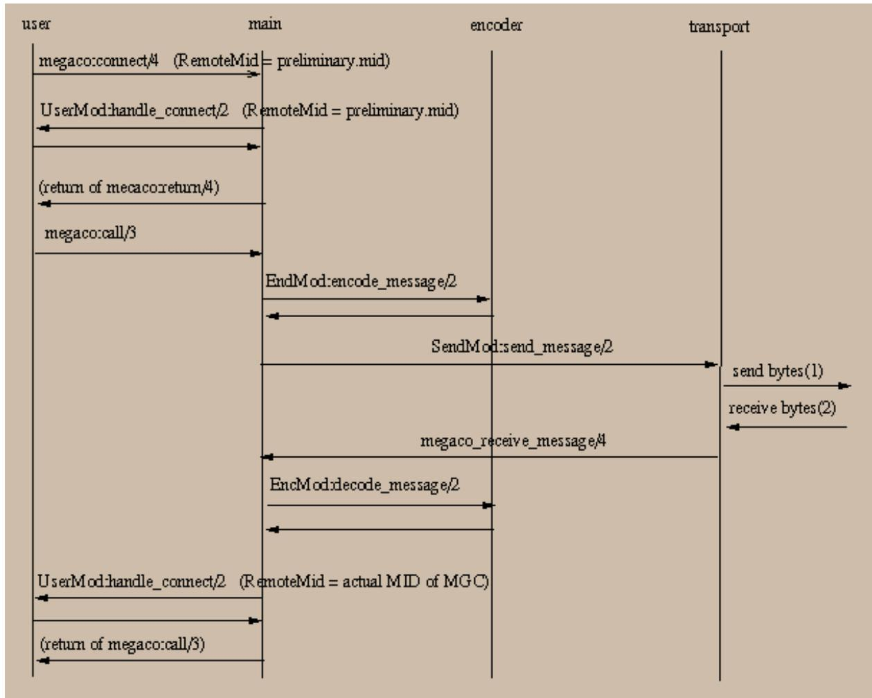
Figure 3.3: MG Startup Call Flow (no MID)
