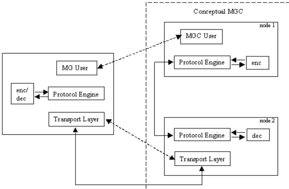
Figure 2.3: Distributed node config
